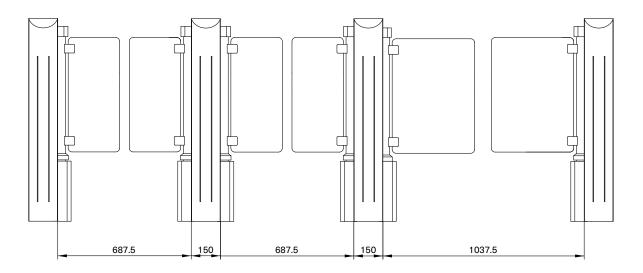
A wide variety of space-saving applications for pedestrians and wheelchair users can easily be implemented using a combination of modules with gates on one or two sides and with narrow or wide passages.
